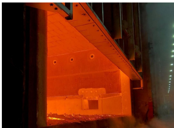
Regenerative forging heating furnace capacity:80m 3
